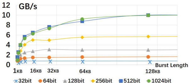
Figure: Effective FPGA DRAM bandwidth
