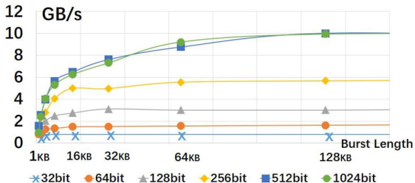
Figure: Effective FPGA DRAM bandwidth
